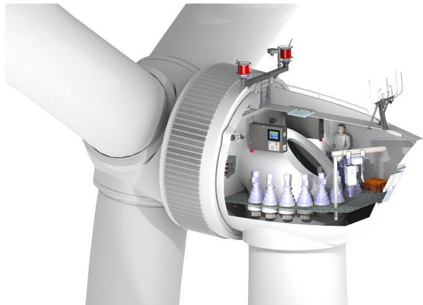
Lagerwey L136-4.5MW platform, nacelle internals
